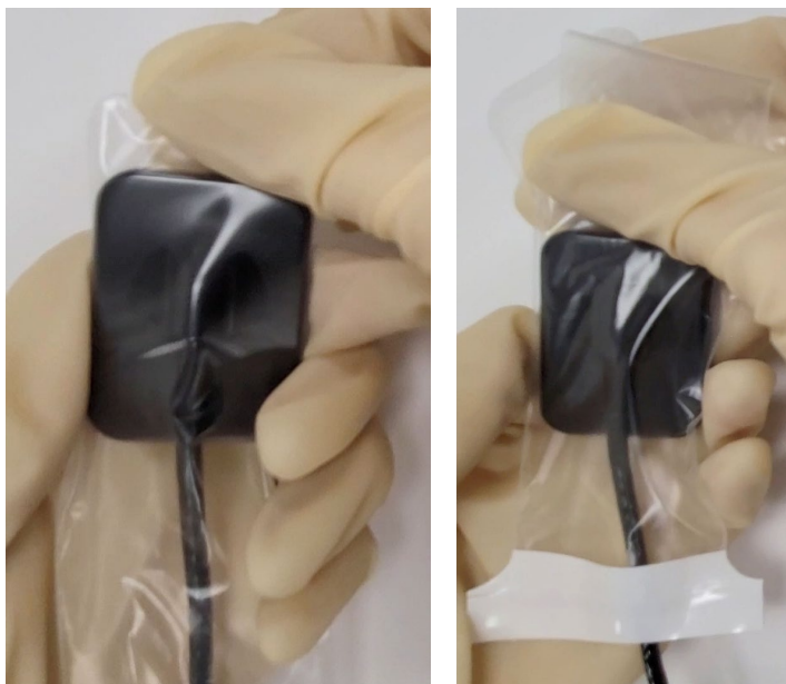
Figures 7. Removing the Sensor from a sheath.
