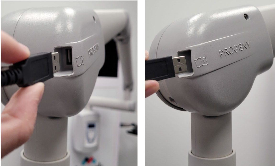
Figures 18. Plugging the Sensor into the USB port on the articulated arm for an integrated system.
